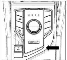
Common function of EPB: static parking / releasing, assistant starting, re-clamping due to high temperature and dynamic parking.
