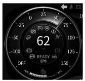
Real-time display of vehicle power (KW)
