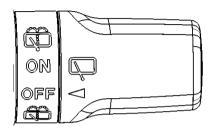
To use washer, upwardly pull the integrated switch of wiper until that the required amount of washing liquid comes from windscreen. Then, the wiper will automatically work for several times.
