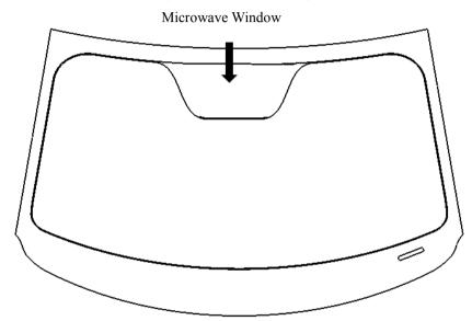
The position of the microwave window is shown in the figure above; and the installation of the electronic identification should meet the requirements of GB/T 35790.1-2017.
