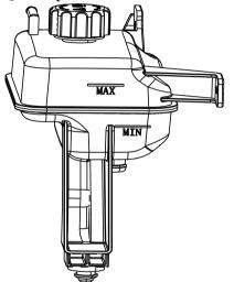
When motor is under cool status, check the level of coolant in tank. If the coolant level is lower than "MIN", please add coolant to the level between "MAX" and "MIN"
