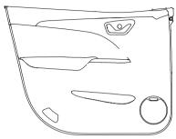
The bottle holders are located at the interior fender apron of four doors.
