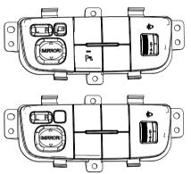
When the switch is set at "ACC" or "ON", the remote control and adjustment are applicable to the exterior rearview mirror.
