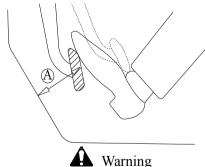
If the brake pedal is too high to back to the normal position, please consult the service stations authorized by DFSK and ask for inspecting brake system.
