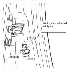
When using the child lock, pull its lock knob toward right to deactivate the inward opening handle, and the doors can only be opened outside the car. Pull the lock knob toward left to release the child lock.
