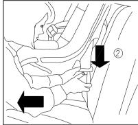
2. Let the seat belt spring bolt go across the child safety seat, and insert to the lock catch ② until feel and hear the locking sound;
