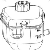
Check the level of antifreeze in tank. If the liquid level of antifreeze is lower than the minimum scale line "MIN", it is necessary to add antifreeze.
