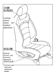
Front Seat - Front Passenger Seat (4-direction Electric Operation)
