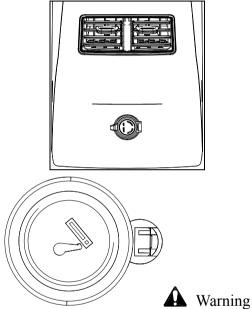
The power of electrical devices shall not be more than 120W to avoid damaging fuse.
