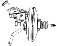
Check the oil capacity in oil tank. If the level is lower "MIN", the warning light of brake liquid will be on, please add brake liquid to the "MAX" level. (Please refer to chapter "Recommended Lubricating Oil and Capacity".)
