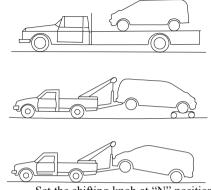
Set the shifting knob at "N" position (neutral gear).
