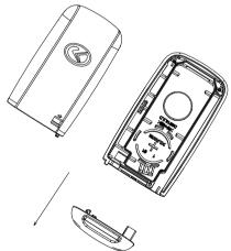
1. Find the button on the back of key, push the button in the arrow direction, and take out the mechanical key in the direction as shown in figure;
