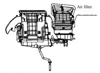
The A/C system is equipped with A/C filter (in HVAC assy.) for removing dirt, pollen, dust or others.
